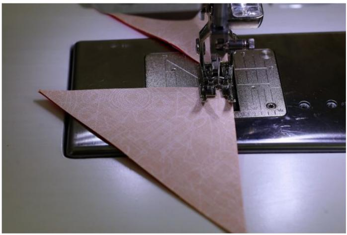
If the points of the triangles seem to scoot out from under the foot, hold them together with a tweezers and guide them under the foot.
